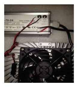
AC Input Side Brown to Line Blue To Neutral. DC Output Side Red and Black To Red and Black from LED Light Green is always to ground.
